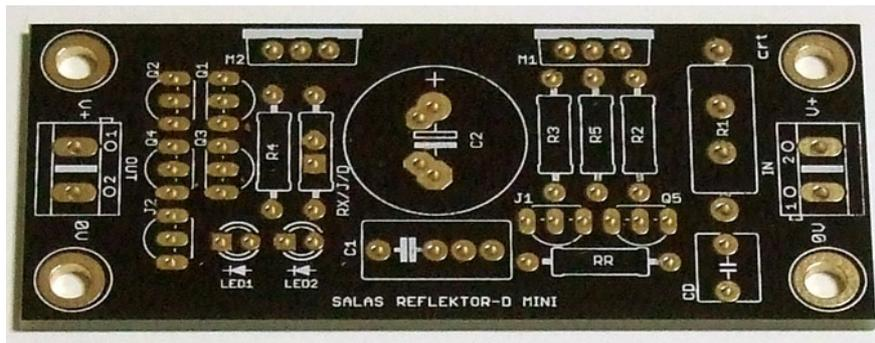
This is a smaller size and simpler version of the Reflektor-D shunt regulator. Meant for where the installation space is restrictive. It does not have own rectification and filtering section and it does not have on board space for sinks. It only accepts DC as input. Has two wire output only. It measures 76mm by 33mm.
