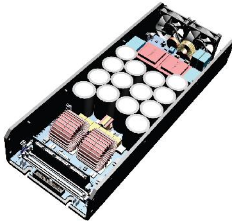
Figure 7 - A 3D drawing view of the dedicated amplifier design.
