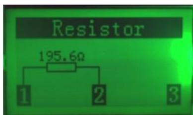
It shows the DUT is an  $195.6\Omega$  resistor, between terminal 1 and 2.
