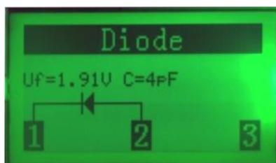
It shows that the DUT is a diode, test terminal 1 is connected to cathode, and test terminal 2 is connected to anode. The forward voltage is  $1.91\text{mV}$ . Junction capacitance is  $4\text{pF}$ .
