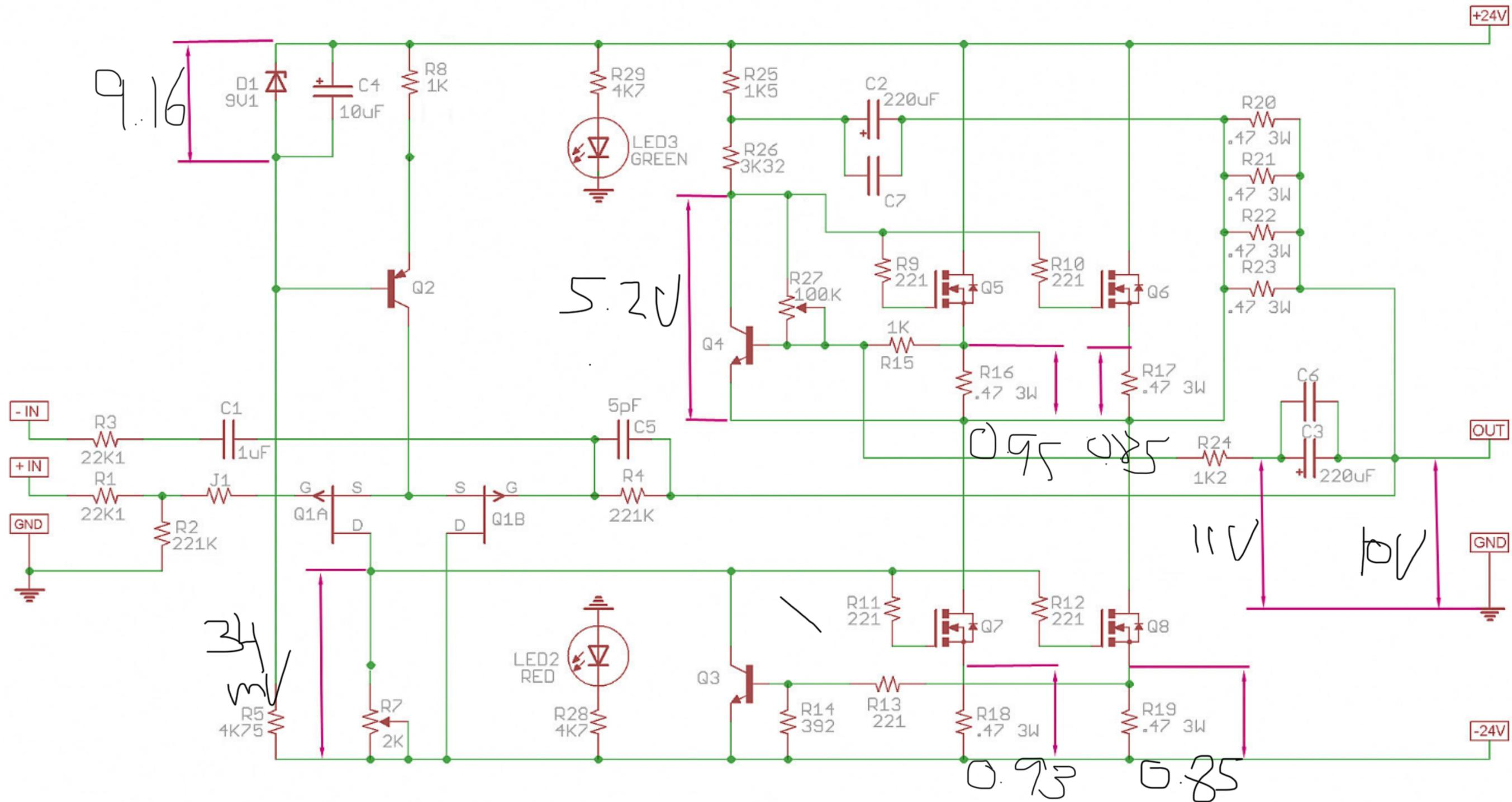
Start with the most basic checks... disconnect the AMP PCBs and confirm that you are getting + and - (20-25V) on the PS PCB.
