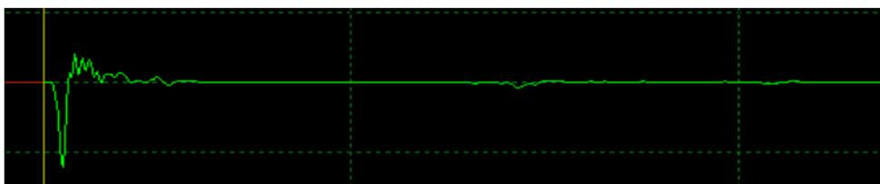
If I gate the measurement to block out the reflection then measurement looks like this.
