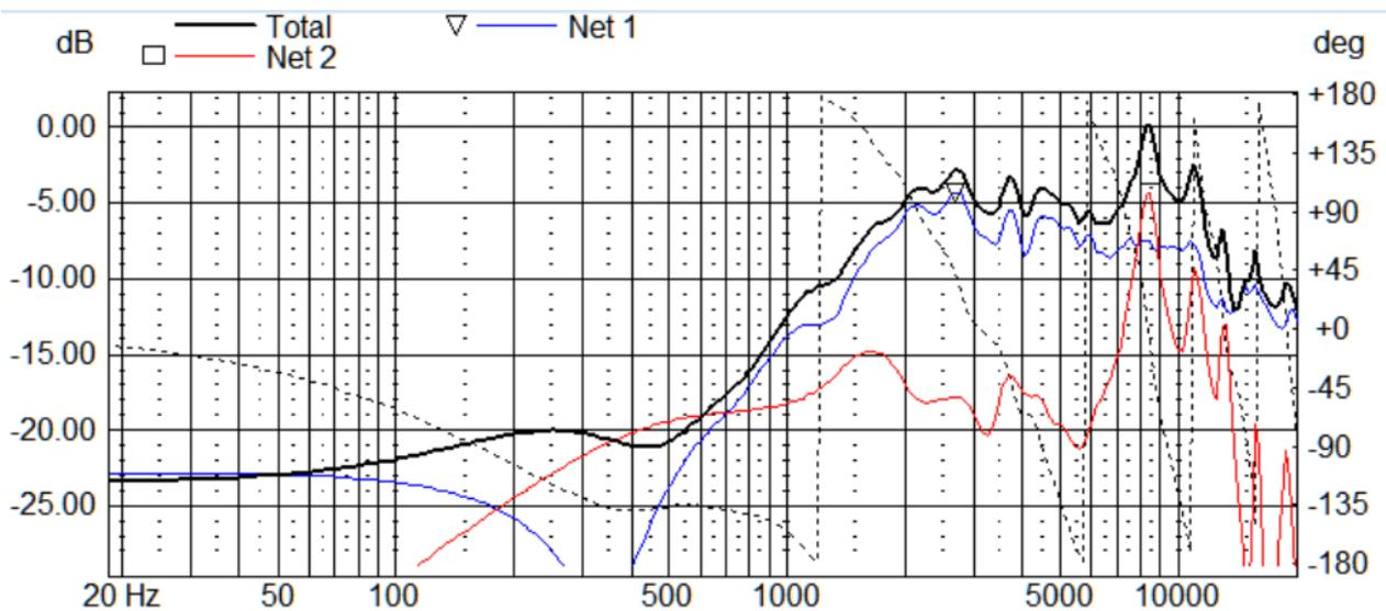
As you can see we've now got the tweeters response (blue) in combination with the mid/basses response (red). The black line however shows what the simulation program has calculated to represent how the two drivers sum together. Now as we actually measured how the two drivers summed before hand, we can now include that measurement and compare the two against one another. When done in LspCAD we end up with something like this.
