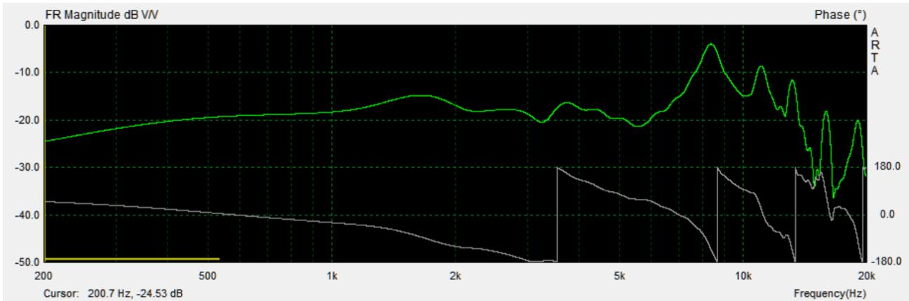
One thing to notice here is the hump at around 1700Hz, this is the standard diffraction bump caused by the narrow cabinet. What you can see however after the bump is the response starting to trail away, this is the start of baffle-step and will be important later on. Export the data.
