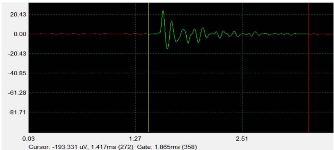
This then turns into the corresponding frequency response graph. It is worth pointing out here that the start point of the gate has to be in the same place, but the end point is free to move around. This is handy because the drivers are mounted in different locations in the room relative to the reflective surfaces and this obviously alters the timing of the reflections incident on the mic. Here I had to shorten the gate by a fraction to keep the first reflection out.
