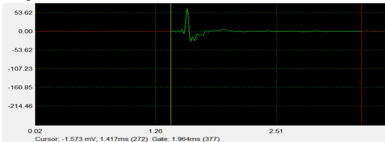
Here we can see that I've chosen a start point of 1.417ms with a total gate length of 1.946ms. This produces the following completely un-smoothed graph.
