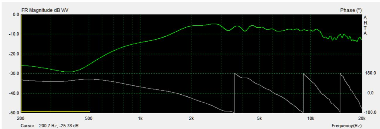
As we can see the relatively short gate only allows us accuracy down to around 500Hz, but as this is miles away from the proposed crossover of around 2kHz it is more than acceptable. The next stage is to export the graph and save it. Don't forget to turn on the phase if it isn't on as standard. Next up is measuring the mid/bass and this is what we get.
