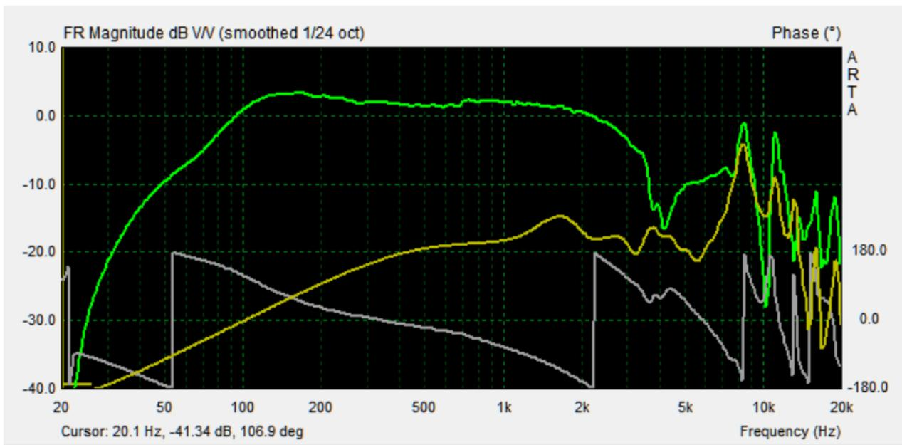
When setting the gate on the near-field response it is once again important to set the start of the gate to 1.417ms.
