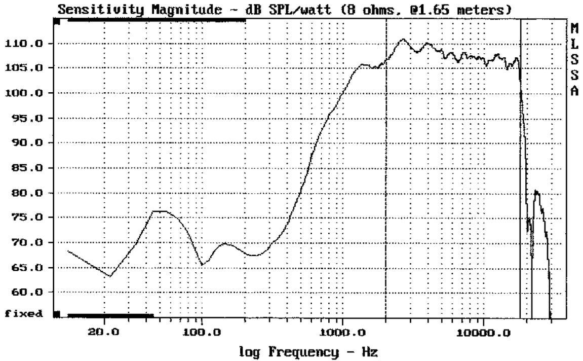
Level (1998:18000 Hz) = 108.08 dB SPL/watt (8 ohms, @1.65 meters)
