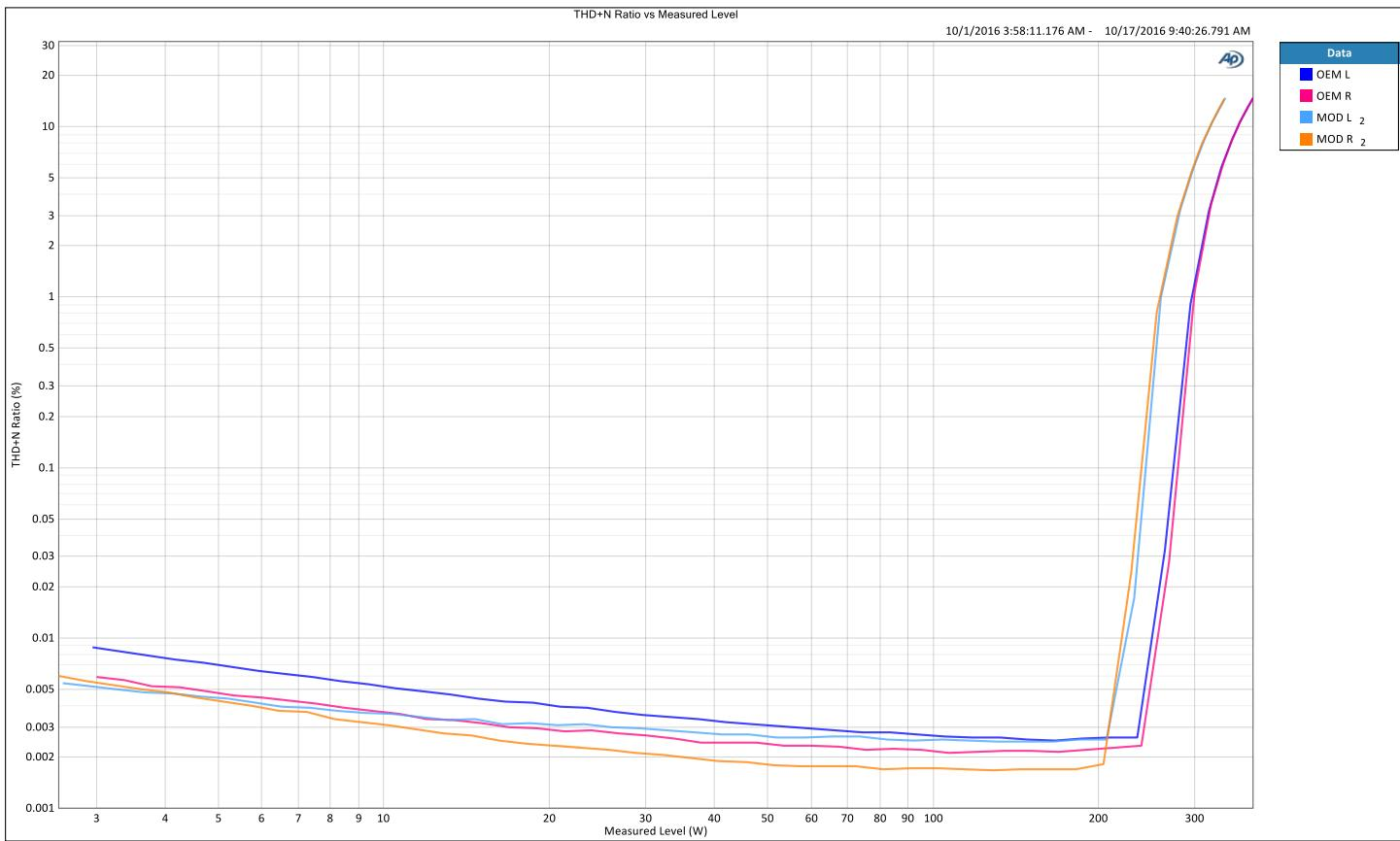
**DC-300A II 10kHz - 20Hz Maximum Output into 4Ω OEM ≈ 0.30V Bias vs. MOD ≈ 0.50V Bias**
