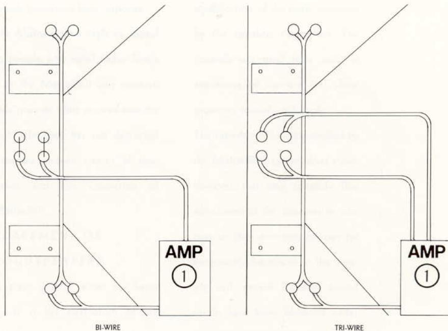
**Bi-/tri-amping.** Ultimately, the use of two or more amplifiers can give further sonic improvements. It is essential, however, that the amplifier gains on each system are very closely matched, in order to maintain the correct system balance.
