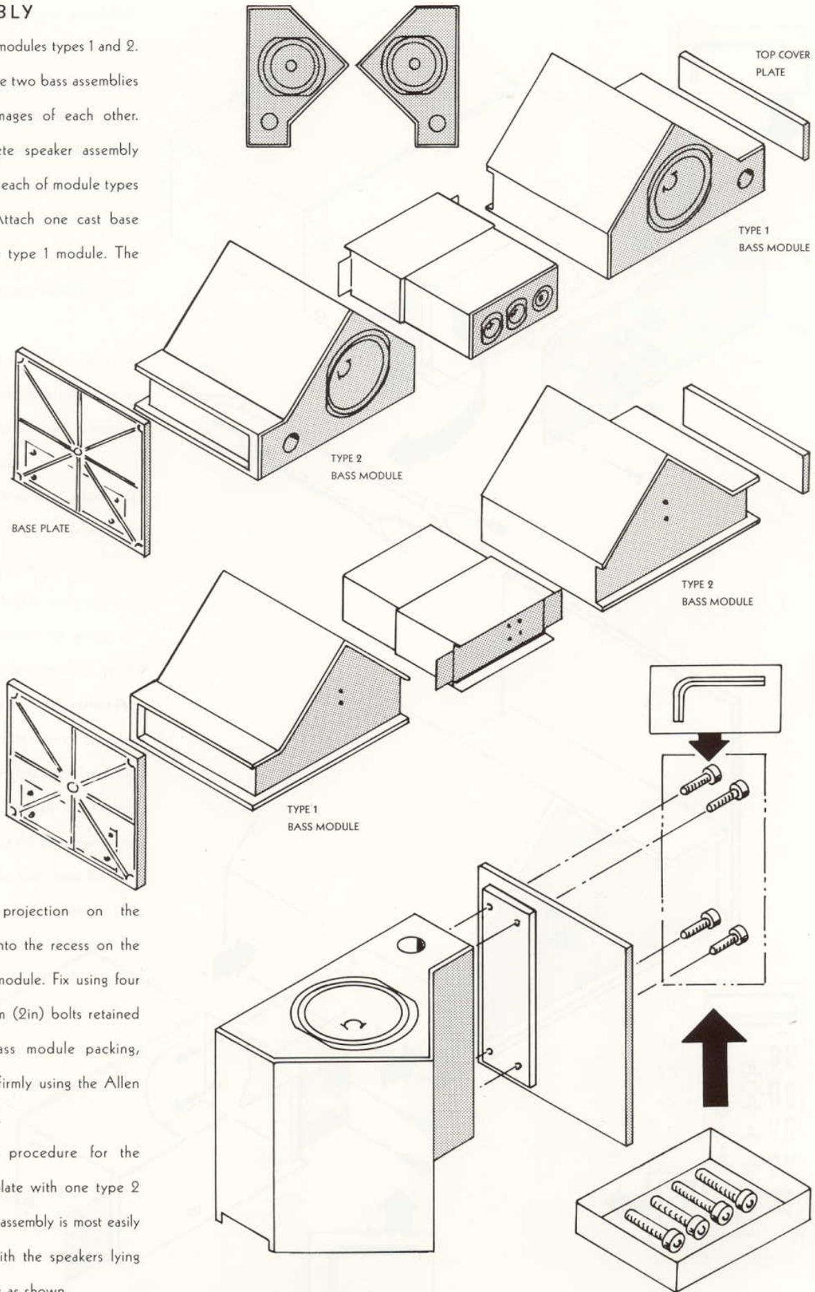
rectangular projection on the casting fits into the recess on the end of the module. Fix using four M8 x 50mm (2in) bolts retained from the bass module packing, and tighten firmly using the Allen key supplied.
