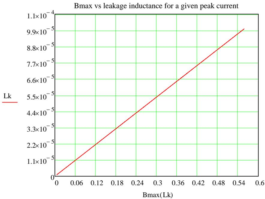
From this chart you can choose a Bmax appropriate for the operating temperature of your CM Choke and see the maximum leakage your design can have at that value of Bmax
