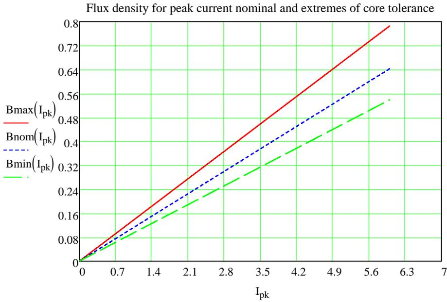
Flux density as a function of peak current. Departure of maximum and minimum values from nominal are a result of core tolerances.
