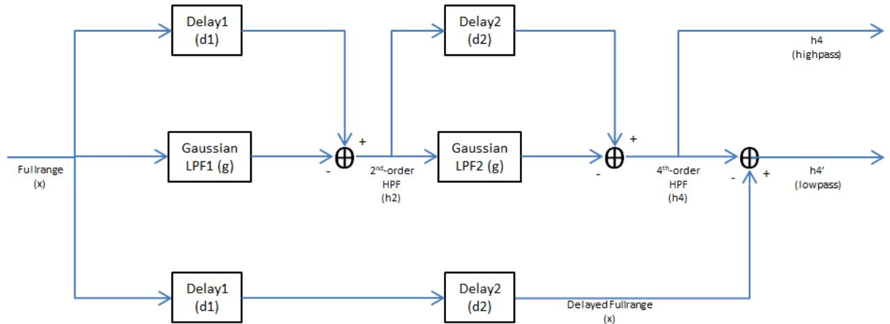
The lowpass filters used for LPF1 and LPF2 are typically, but not necessarily, Gaussian or Bessel.
