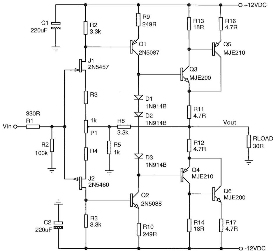
Figure 8: The complete headphone amplifier/buffer.
