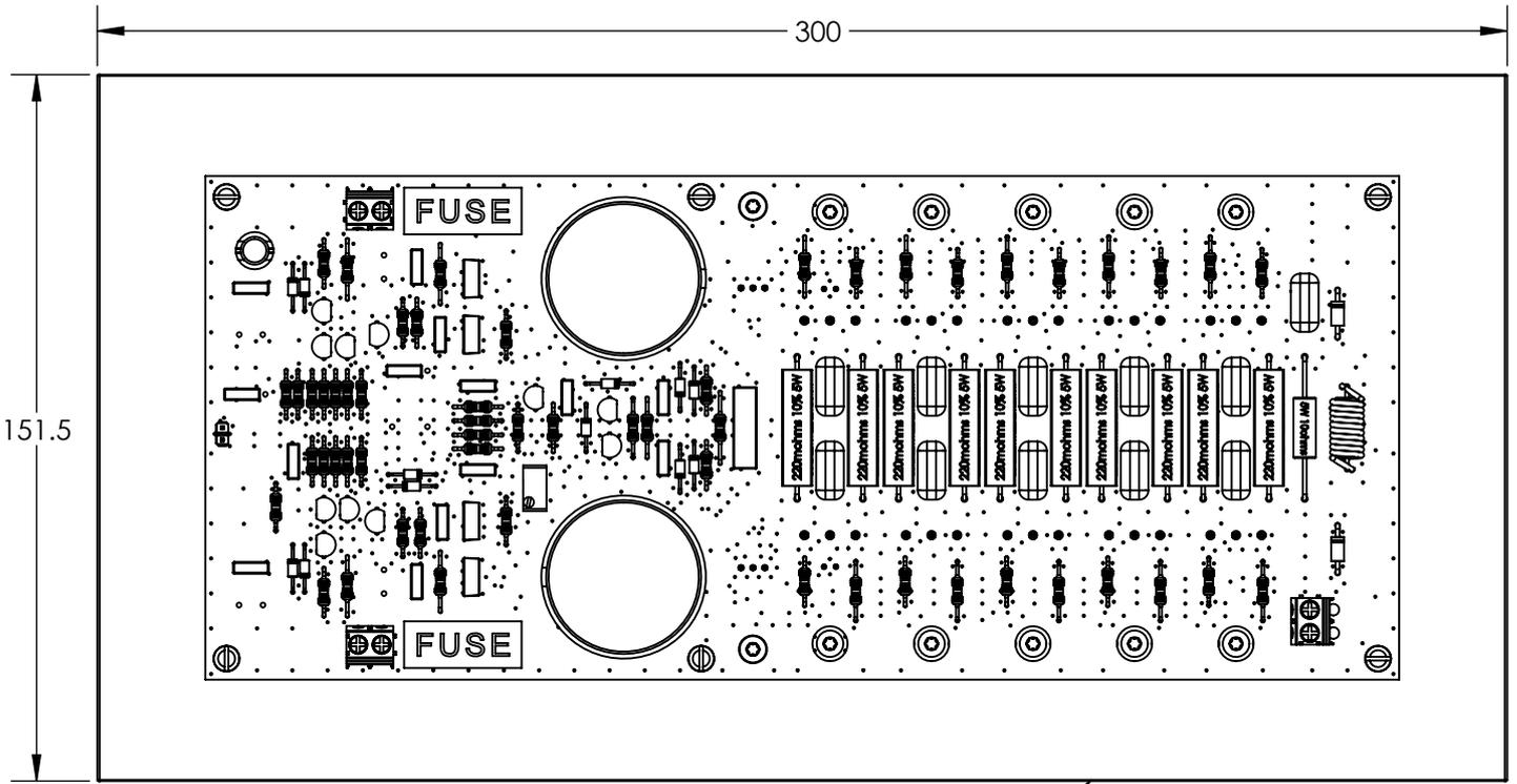
Example based on Conrad Heatsink model MF30-151.5 Flat Back
