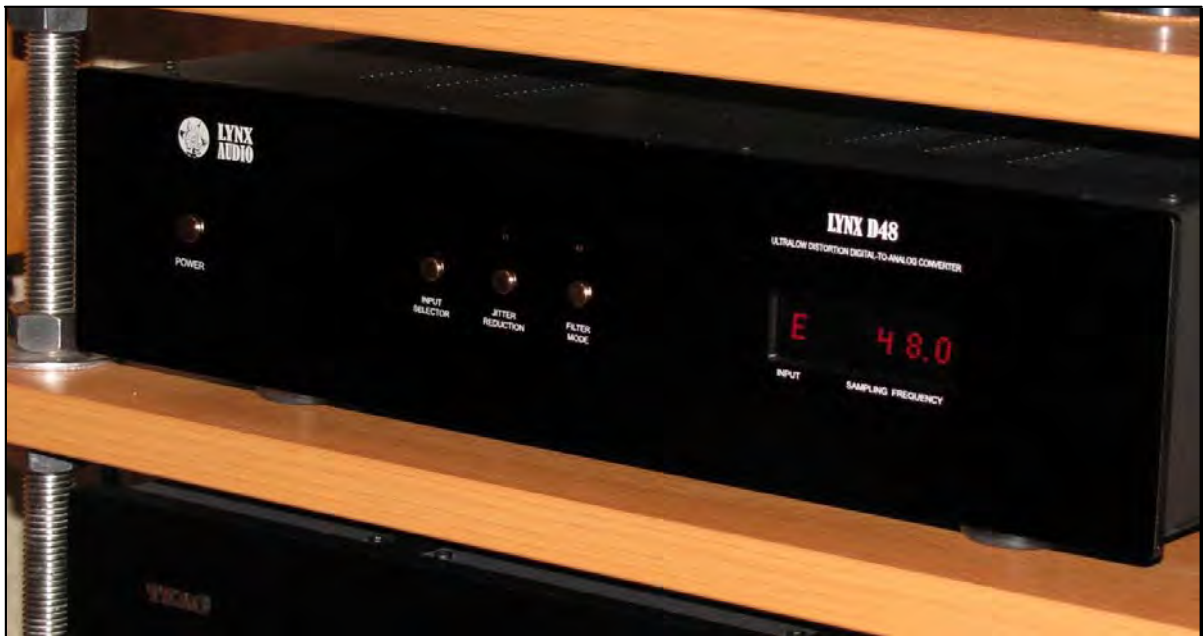
Fig. 10 Finished DAC block based on Lynx D48V3 module
