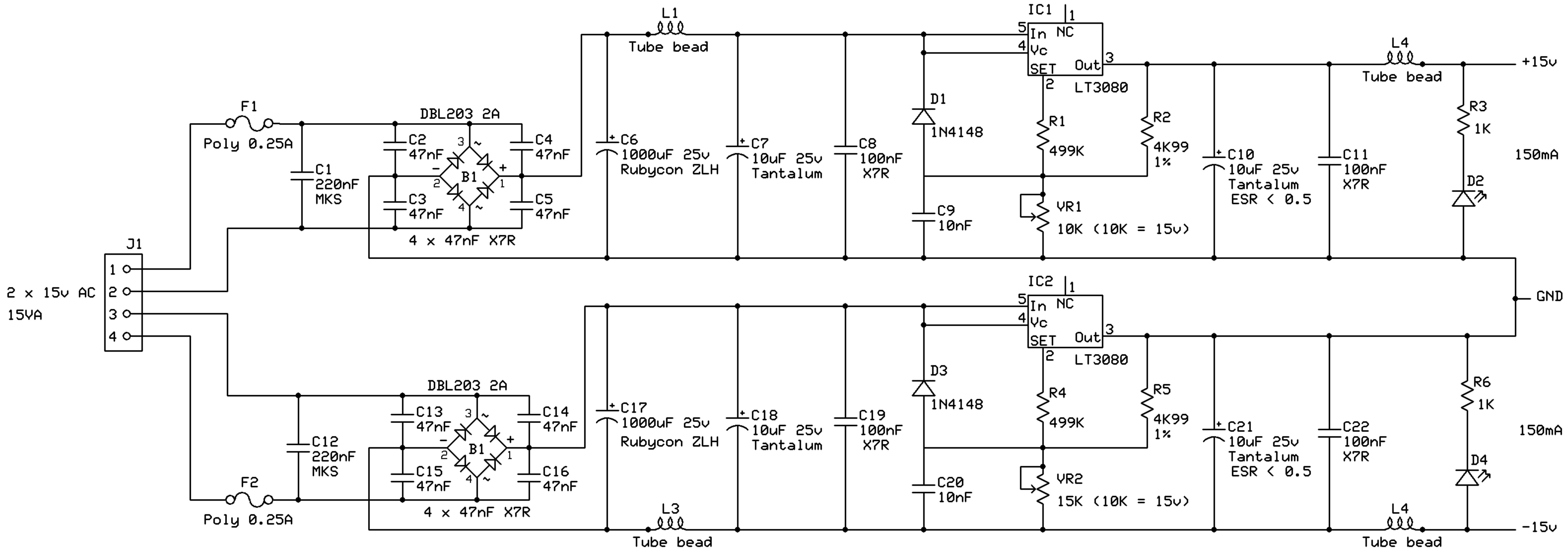
C9 and C20 : Try values between 10nF and 1uF (max 1uF)
