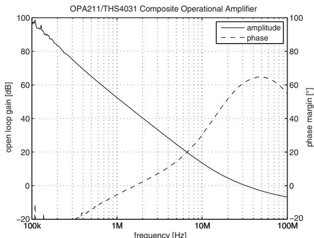
Fig. 2. Measured open-loop gain for the proposed composite operational amplifier.
