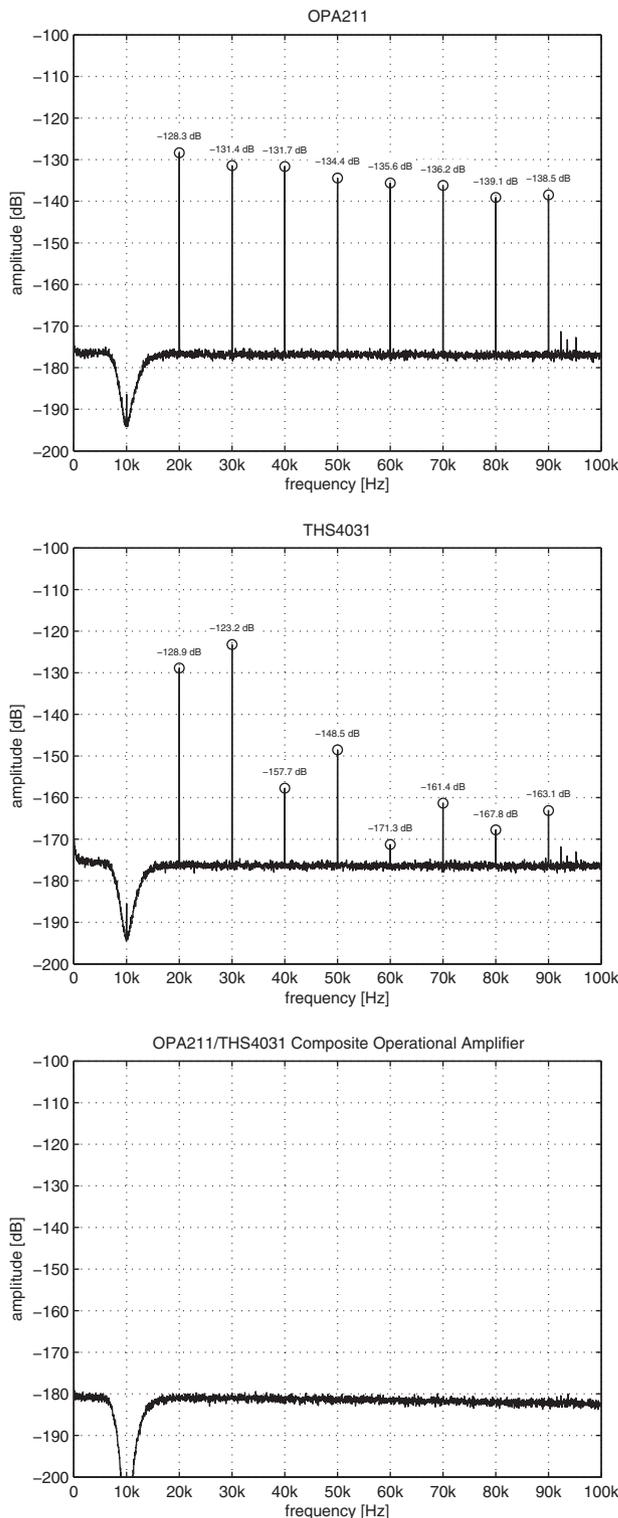
Fig. 3. Measured input-referred harmonic distortion voltage at 10 kHz for the OPA211, THS4031, and resulting composite operational amplifier.
