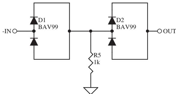
Fig. 4. Clamping network connected to  $U_1$ .
