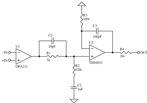
Fig. 1. Proposed composite operational amplifier.
