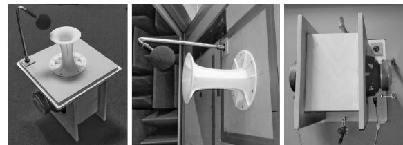
Fig. 7: Photos of test box with two 10-inch woofers and microphone fixture. Left: Box before mounting. Middle: Box with port mounted inside hemi-anechoic chamber. Right: Box mounted to hemi-anechoic chamber wall, shown from outside.
