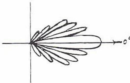
**A "medium-priced", minimum-phase, closed-box loudspeaker (A standard DAL model) at about 3 KHz**
