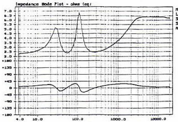
A "medium-priced", minimum-phase, closed-box loudspeaker (A standard DAL model)
