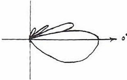
**A highly-rated, "medium-priced", planar membrane loudspeaker at about 3 KHz**
