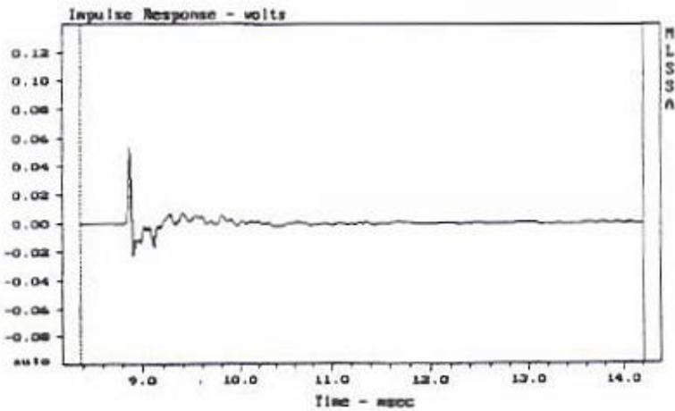
A "medium-priced", minimum-phase, closed-box loudspeaker (A standard DAL model)
