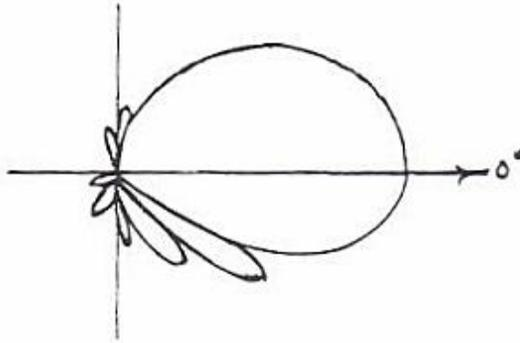
**A highly-rated, "medium-priced", planar membrane loudspeaker at about 3 KHz**
