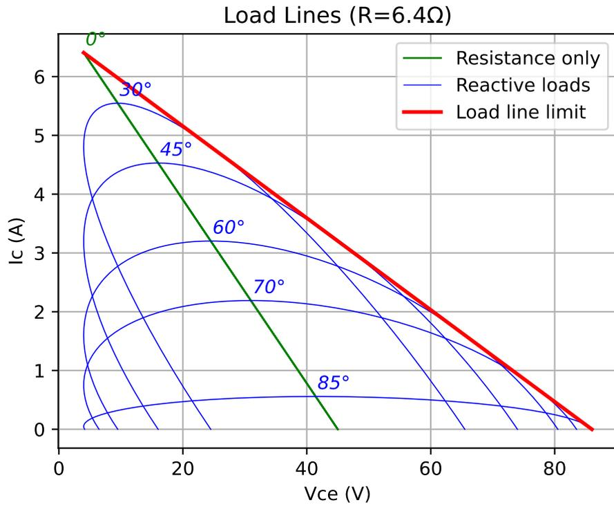
These load lines are a good match for the results presented in Cordell's book. The nonlinear behaviour as  $I_c$  approaches zero is not captured, but this is not relevant for load sizing. There has been no provision for an emitter resistor. This could be included if necessary. I believe the results presented by Cordell are obtained by extracting values from a spice simulation of an amplifier.
