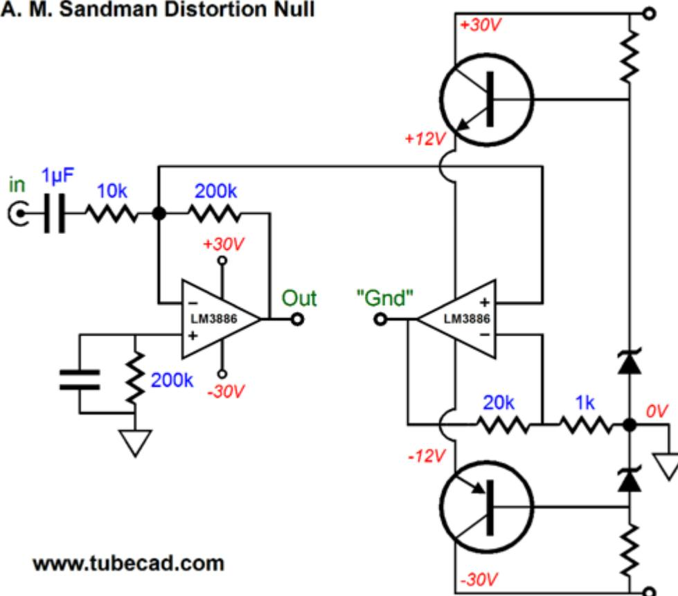
This solution would limit the heat the error-take-off amplifier would produce, but it also limited the potential power output that the two amplifiers could deliver into the speaker. Remember that the error-take-off amplifier's output voltage hovers around 0V as long as the main power amplifier does not clip.
