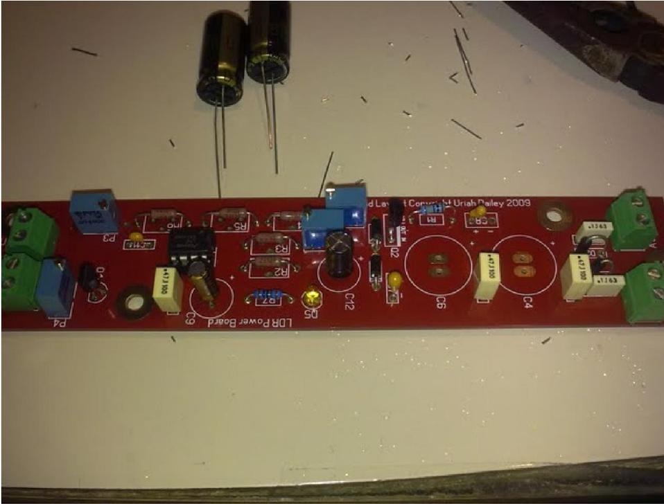
All trimmers and .47uf caps in place as well as 47uf near opamp and 100uf near LM317.
