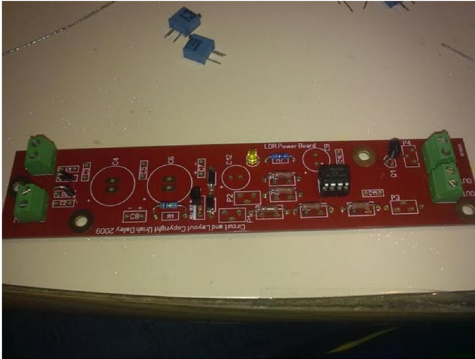
Terminal blocks in. Should have put them in first but I learned the hard way. Note the diodes. Its easy to fit them this way. You can actually get them to fit perfect but its a 90degree angle down from the body of the diode and sometimes thats hard to bend perfectly.
