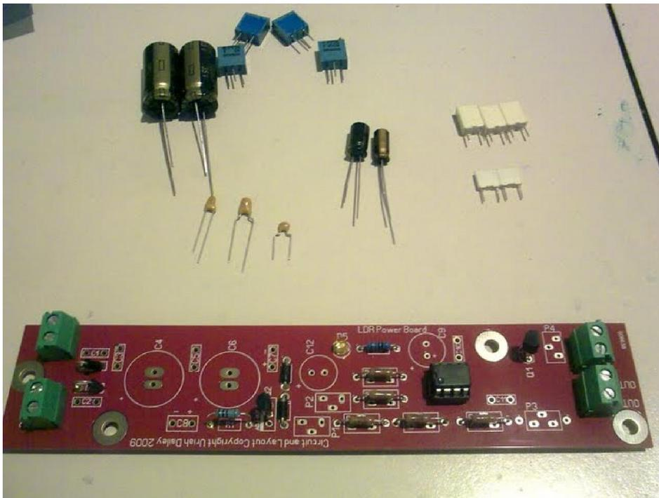
See those little yellow guys? Left one is .1uf. Middle one but largest is 1uf. Small one on the left is 68pf. The large electrolytics are 1000uf as marked and then you have two other electros at 100uf and 47uf. The white boxes: the 3 larger ones are .47uf and the two smaller are .1uf.
