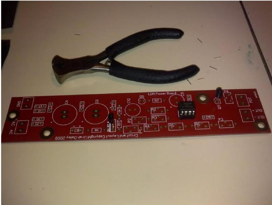
Trim the legs after soldering. See the dimple on the LME49710? Yes in this photo I have LM334 in with the pin 2 and 3 in the wrong holes. Remember your tubing. Remember to reverse those legs.
