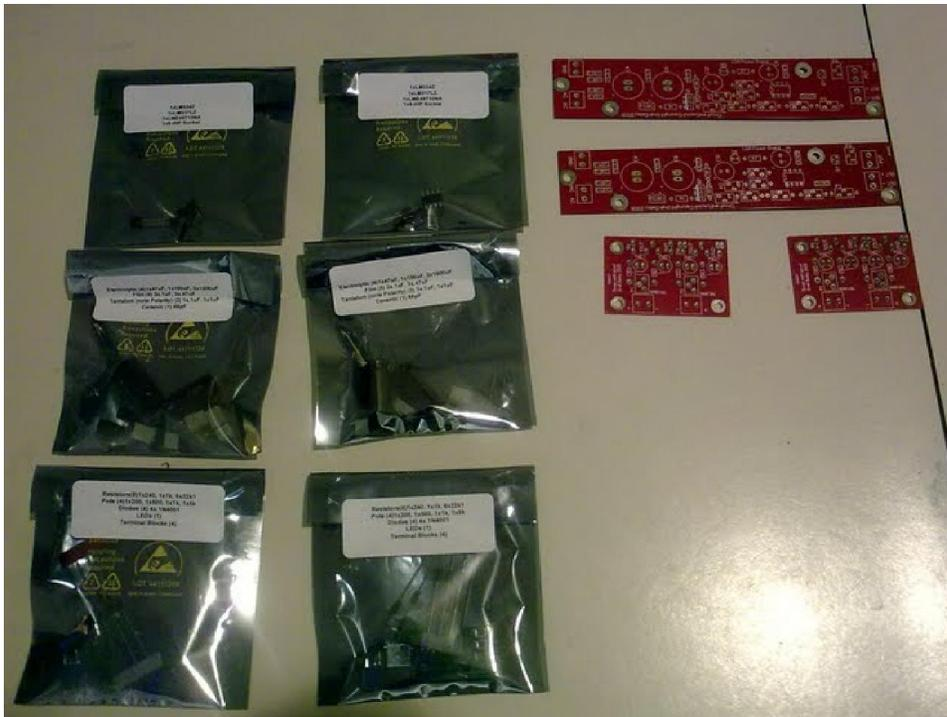
2 LDR controller boards, 2 BOM, and a mount and balance board. 2x Mount Balance shown, only 1 needed.
