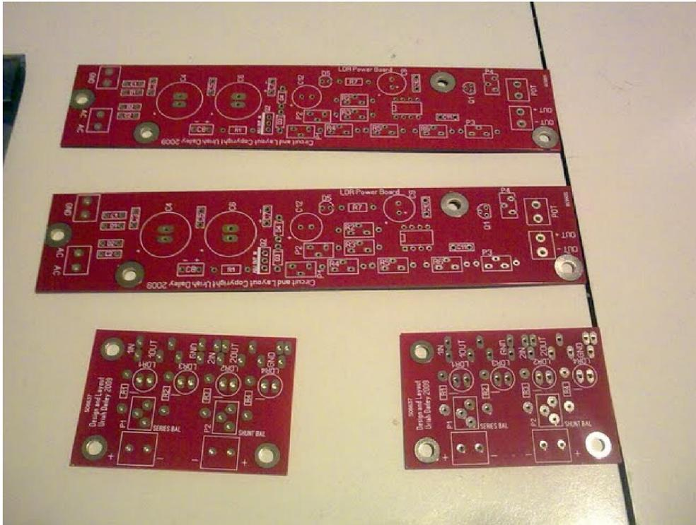
Close up of the boards. Starting with the top boards, the LDR Controller boards...
