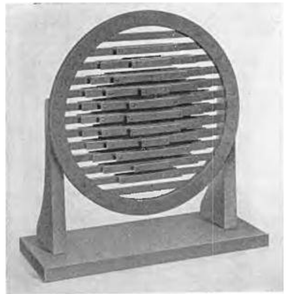
FIG. 12. A double convex strip lens 10 in. in diameter. The strip size and spacing is the same as that used in the prism of Fig. 9.
