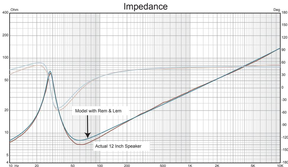
The graph above now shows the results using the new motor impedance model. There is substantial improvement. Both the magnitude and phase match very well across the entire three decades of frequency. The maximum error of 1.1dB occurs near 60Hz. The four coefficient values used are:
