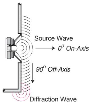
These parameters greatly affect the diffraction modeling of enclosures. For transducers which are surface mounted, the sound wave radiating towards the edge of the enclosure results from the 90 degree off-axis radiation of the transducer as shown here in the pictorial.
