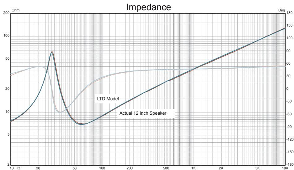
Since the acoustic response is very much dependent on the impedance response, the improvements in the motor impedance model should facilitate similar improvements for the simulation of acoustic response.
