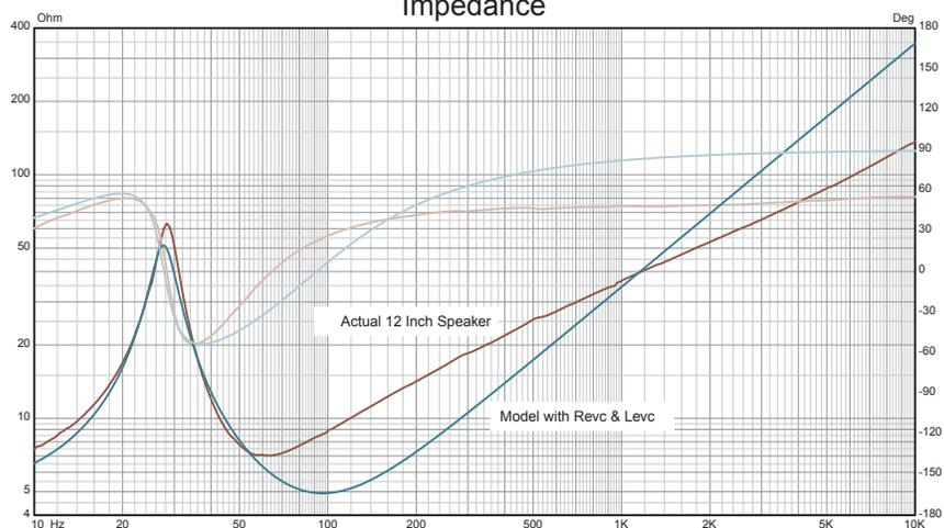
The previous model using  $Levc$  corresponds to the **STD** model in *EnclosureShop*, and is the old traditional method for transducer modeling. This model produces an error of nearly 6dB at 100Hz.
