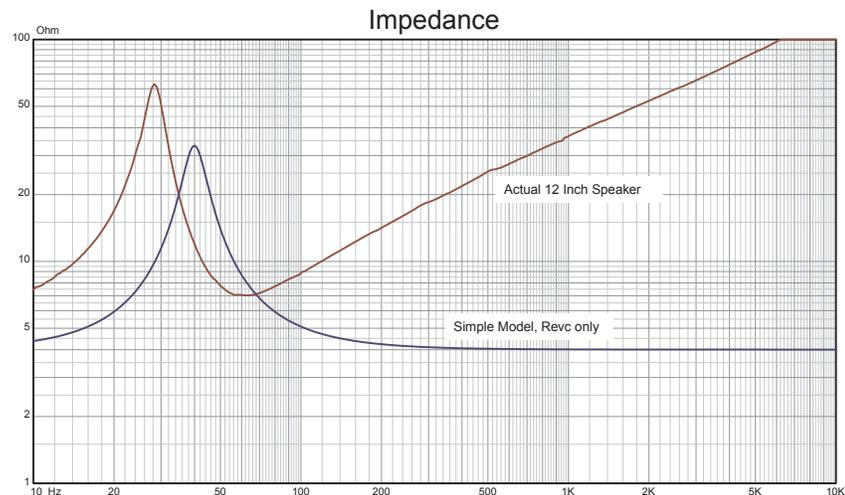
The rising impedance of the actual transducer has the obvious appearance of inductance. It would seem that adding an additional inductor component  $Levc$  would be a logical approach. The electrical circuit for a free field transducer is now shown below with the additional component  $Levc$ . The relationships for the mechanical components are also shown in the equations to the left.
