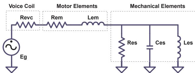
The circuit here shows a new arrangement for the electrical circuit, and two new components:  $Rem$  and  $Lem$ . These two comprise the *motor impedance*. Both are frequency dependent.
