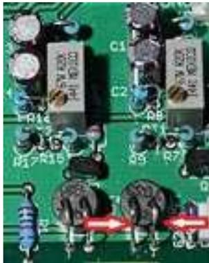
3. Adjust the trimmer corresponding to each LDR (trimmer "RT1" corresponds to LDR "LSE", "RT2" to "LSH", "RT3" to "RSE", "RT4" to "RSH") until you measure around 700Kohm. The precise value is not critical, but it should be between 500K and 1M.
