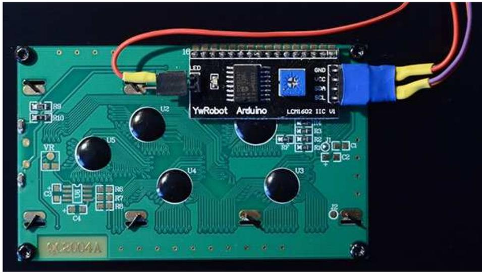
The backlight wire "LCD LED" goes to the upper pin of the "LED" header on the LCD module (remove any jumper, if present).
