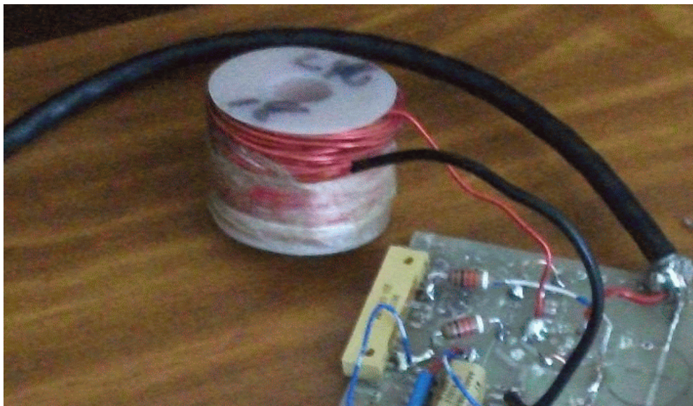
This Coil is an AIR-core Type – Hi - “Q” type.
