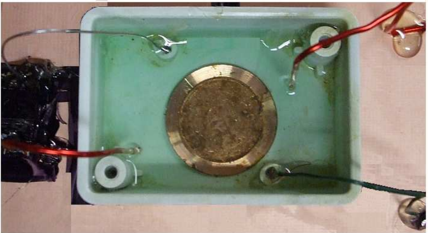
Sealed LM733C Op-Amp. : Cu-Disc, CuSo 4 , Iron & Copper wire
