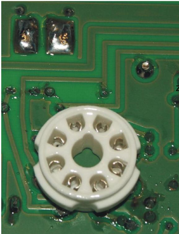
Another photo with soldered z pad and soldered pin 2 + 7
