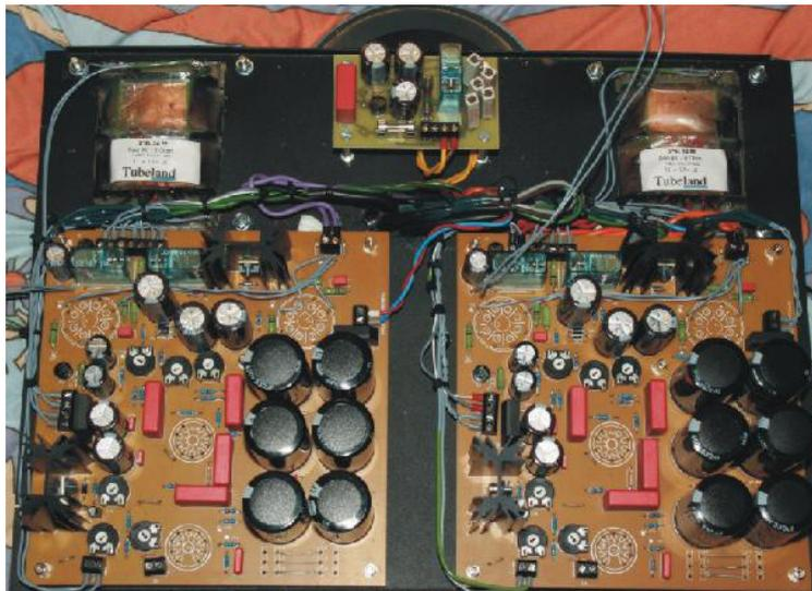
Install the lead to the switch for pentode operation. Then install everything and wire it to each other. As a craft pad, something soft to take to avoid scratches would be good.
