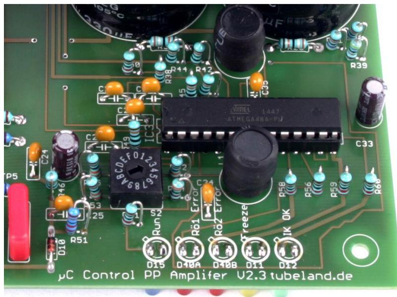
The picture shows again the DIP switch position for the KT88 Amp level 3-4 is correct here!
