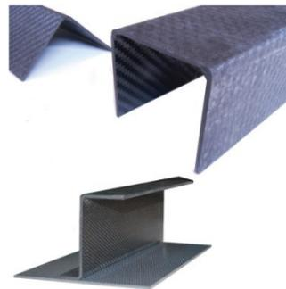
**THERMOFORM** advanced composite sheets can be formed into shaped parts with the application of heat and pressure. Our formable composite sheets can consist of carbon, glass or aramid reinforcements. These products can be over-moulded, joined together with fusion welding techniques and are more readily recyclable.
