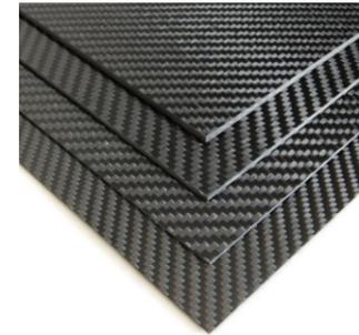
**STANDARD** carbon fibre sheet is manufactured using multiple layers of genuine 100% carbon fibre infused with epoxy resin creating a high stiffness, high strength, light weight and aesthetically pleasing material. All STANDARD carbon fibre sheets have a glass transition temperature of 90°C with higher temperature performance available upon request. Other sizes and thicknesses available upon request.
