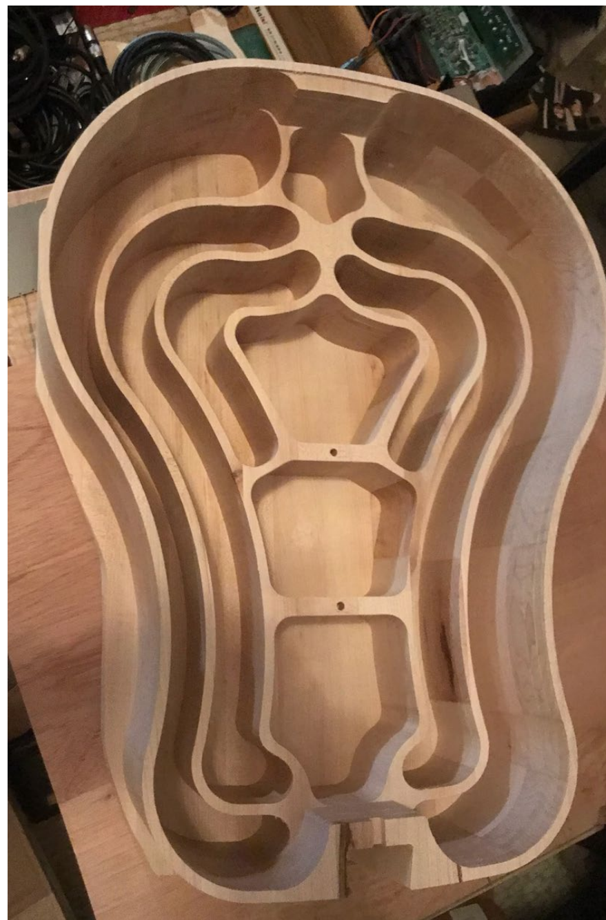
Jig sawed the excess wood off.
