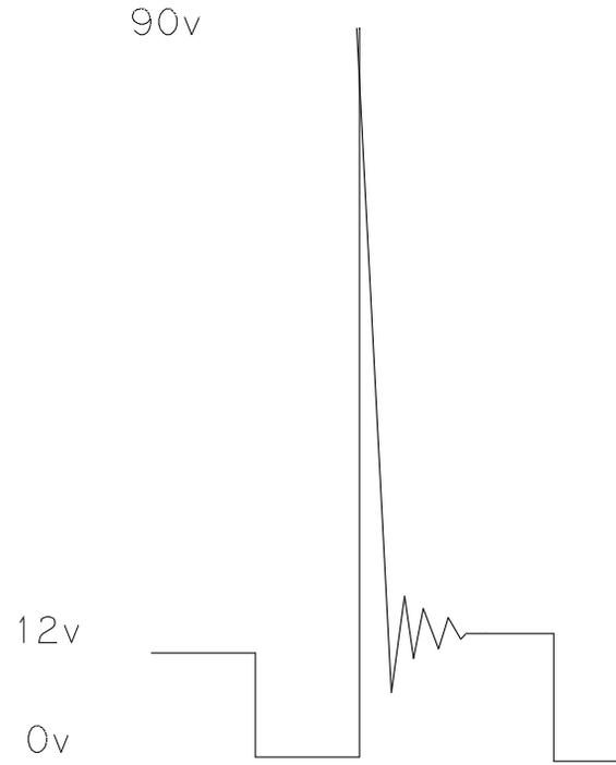
measured at source drain of either side of transformer
