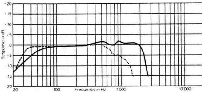
Frequency response contour of the 2245H taken in a hemispherical free-field environment, a closed box of 280 L (10 ft³) internal volume enclosing the rear of the driver. Measured response of a typical production unit, including all peaks and dips, does not deviate more than 2 dB from the above curve. The dashed curve represents the response from a 320 cm² (50 in²) port with a 20 cm (8 in) long duct tuning this enclosure to 30 Hz.
