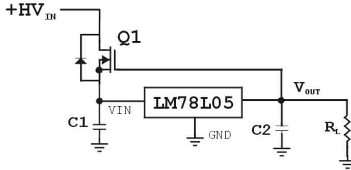
Figure 10: High Voltage Off-line Linear Voltage Regulator [2]
