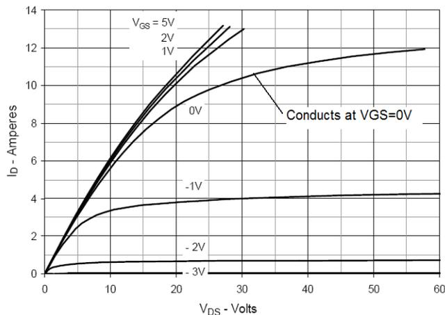
Figure 2: Output characteristics of N-channel Depletion-mode power MOSFET
