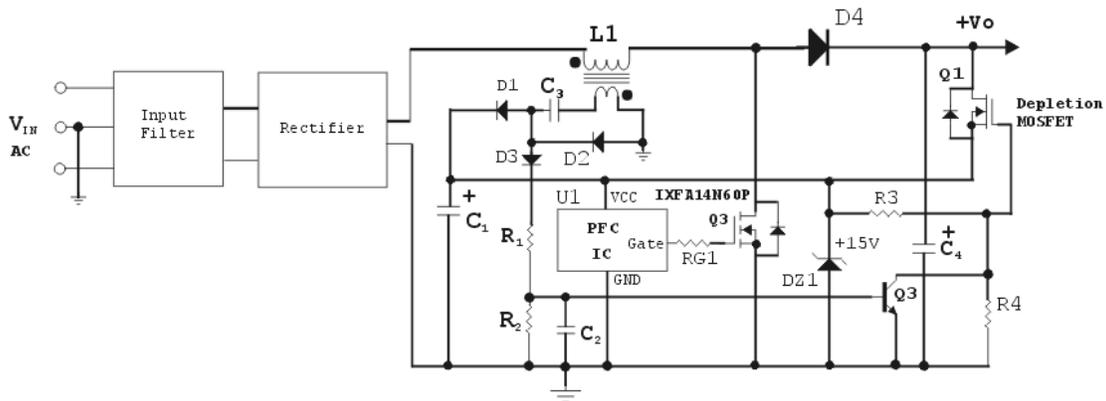
Figure 7: Power Supply start-up circuit using Depletion-mode MOSFET [3]
