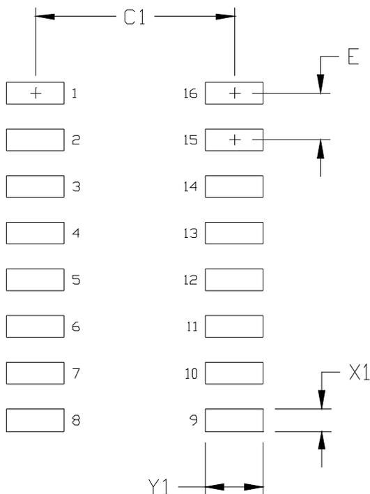
**Figure 19. 16-Pin Narrow Body SOIC PCB Land Pattern**
