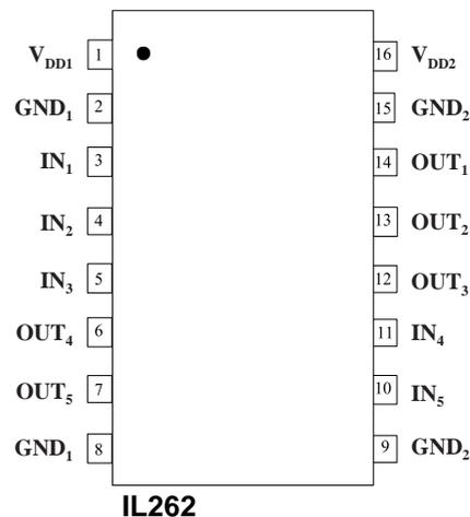
\*NOTE: Pins 2 and 8 are internally connected, as are pins 9 and 15.
