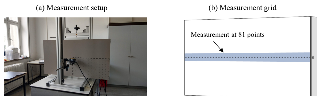
Figure 13. (a) Measurement setup with a Keyence HK-052 laser at the Technical University of Dresden. (b) Overview of the measurement grid: 81 points on the central line are measured.
