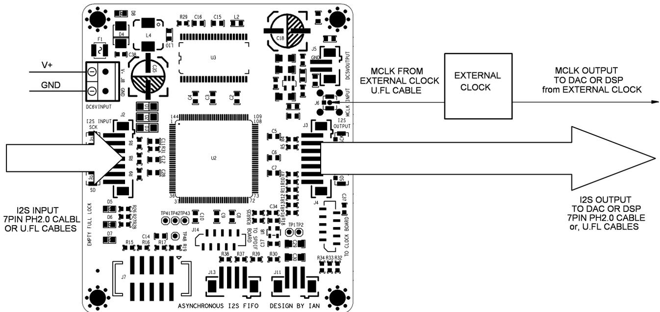
If this configuration is really needed, it is highly recommended to connect the external clock directly to the XO socket on the clock board. For external clock, the logic level of MCLK input on the I2S FIFO Board must be LVTTTL (3.3V) and the MCLK frequency must be fixed at  $256 \cdot F_s$ .
