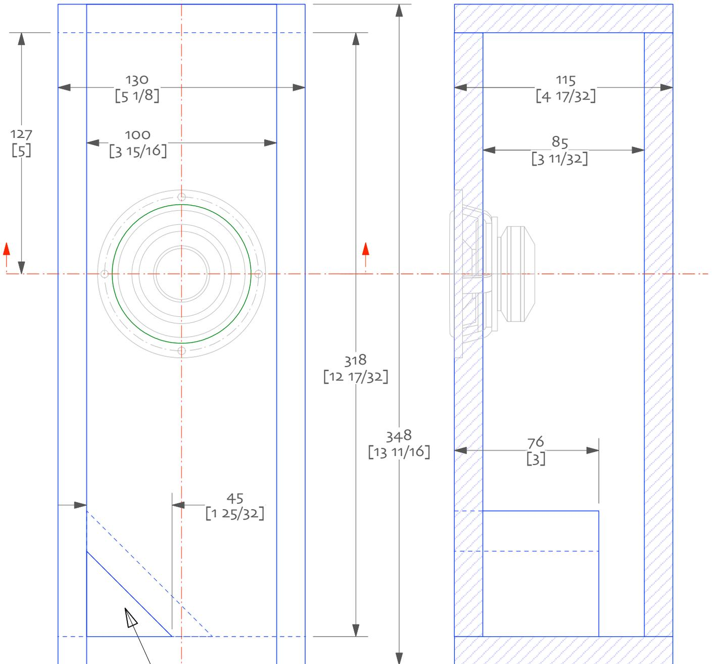
alternate vent is 10mm high, width of box
