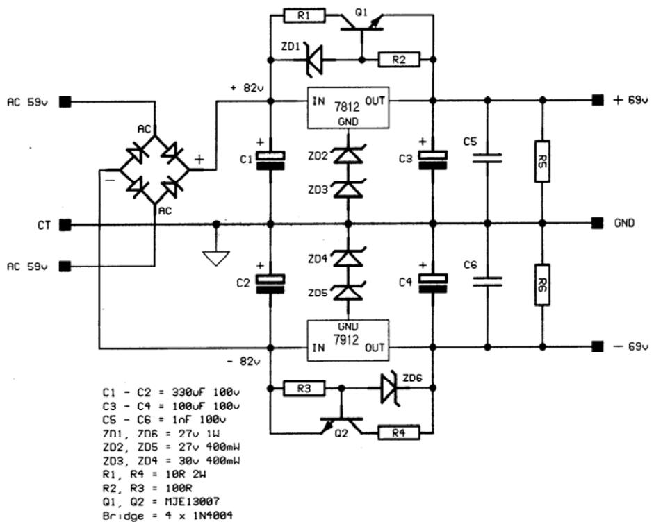
Zener diodes ZD2 - ZD5 set the voltage for the regulator output, i.e.  $27 + 30 + 12$  (reg) = 69 volts.
