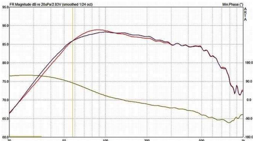
This graph shows the filtered response of the woofer in the 24 liter closed cabinet of the Black Box. The red curve is without the woofer series capacitor, the purple curve shows what happens when a large capacitor is placed directly before the woofer - all other crossover components are unaltered. The bump in the octave from 60-120Hz is lowered and there is a little boost from 120-300Hz
