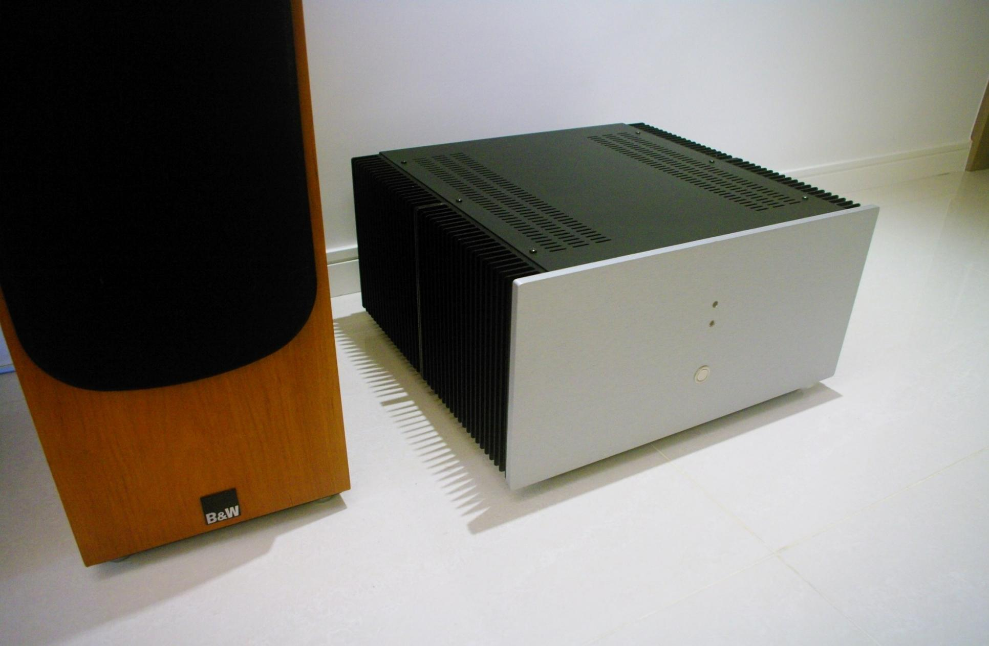
180 W RMS per channel [‘e-Amplifier’](#) featuring VFA topology, 10ppm 20 kHz distortion and peak output currents of  $\sim 40A$ , 3 Hz to 200 kHz bandwidth, and better than -100dB noise and hum ref 2.8V peak output into 8 Ohms that uses the wiring techniques described in this document.
