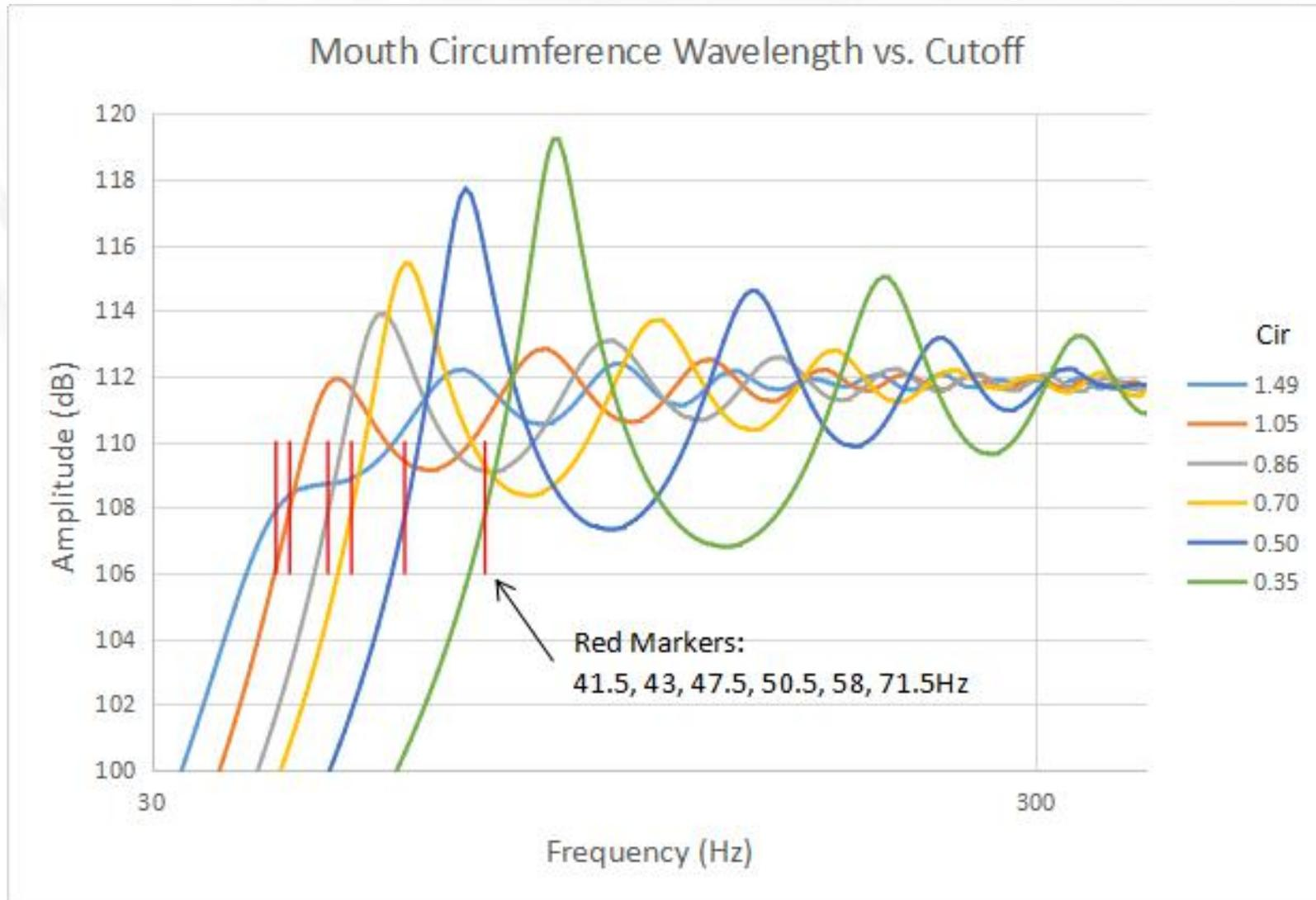
The horn cutoff frequency does not change much from 1.0 to 1.5 circumference wavelengths (CW).
