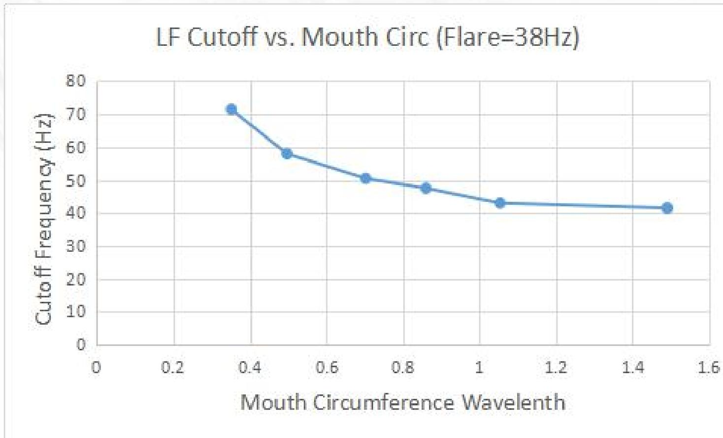
From a ripple standpoint, there is not much difference between 1.0 and 1.5 CW. The curve slope is linear with mouths smaller than 1.0 CW.
