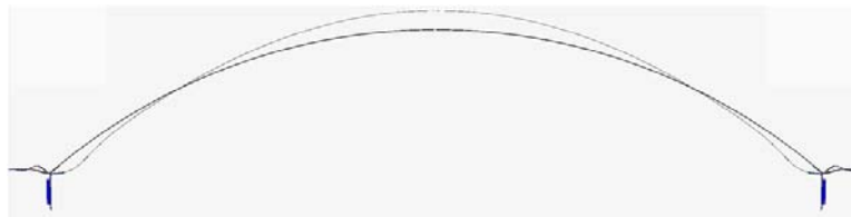
Figure 1. 2D Mode Shape at 1 st Bending Frequency of a Dome Diaphragm.
