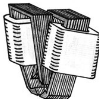
"POLE PIECE STACK" ASSEMBLY
