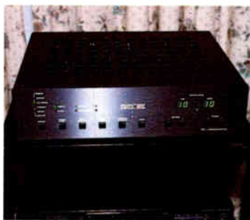
Joule's Electra LA-100 (above), a valve line pre-amp, contains MIT caps and Cardas wiring
