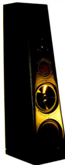
Thiel CS7 (right) has a 65lb cast concrete baffle on which the drivers, including a 12 in aluminium cone woofer are robustly mounted
