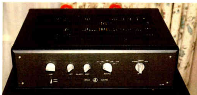
Joule's Electra LA-100 (above), a valve line pre-amp, contains MIT caps and Cardas wiring
