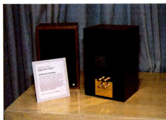
Thiel CS7 (right) has a 65lb cast concrete baffle on which the drivers, including a 12 in aluminium cone woofer are robustly mounted
