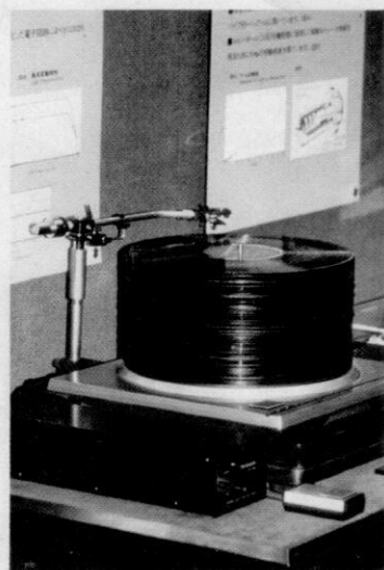
ABOVE: Not a multi-changer version but a demo of the powerful motor torque
