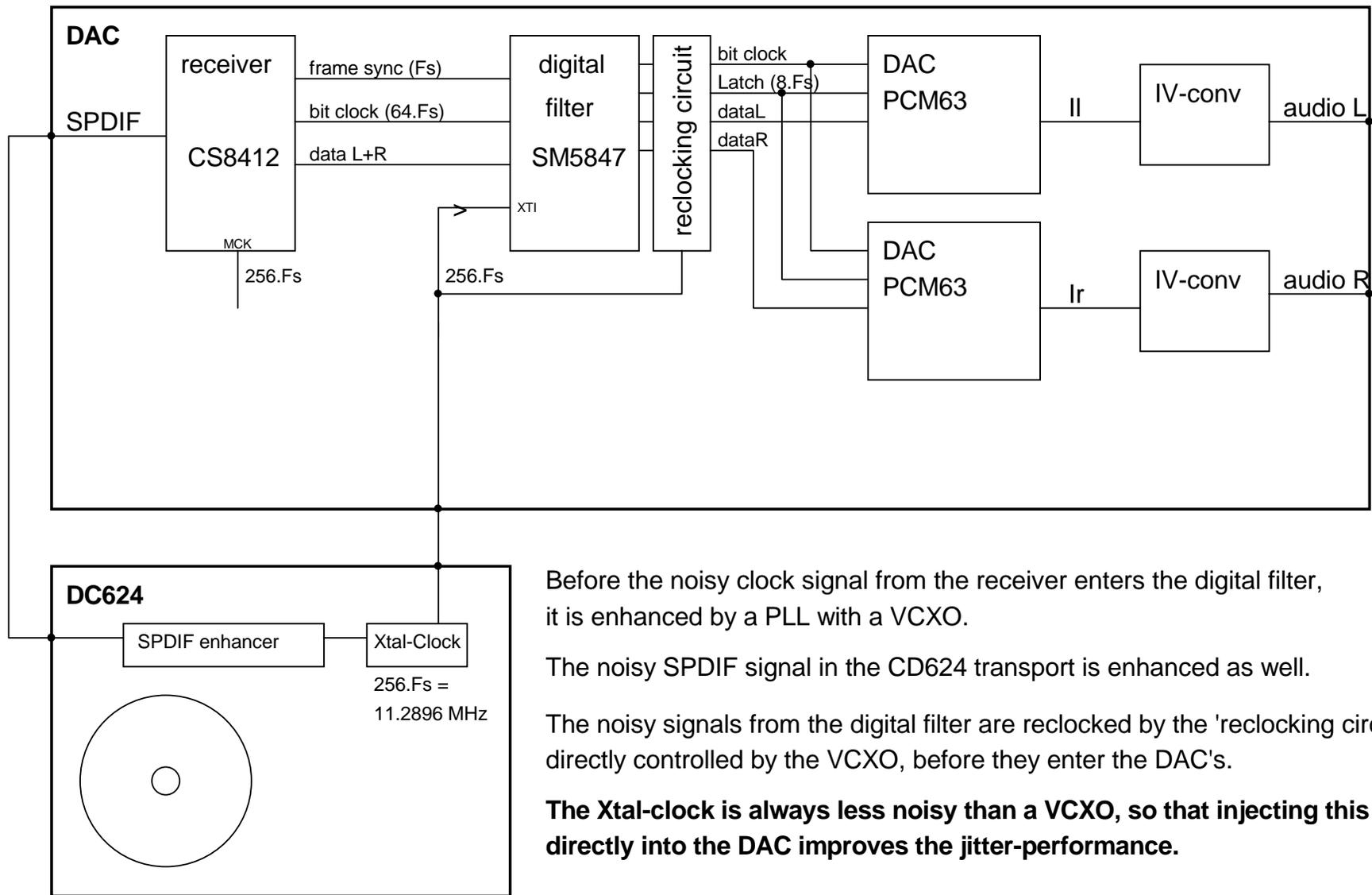
Before the noisy clock signal from the receiver enters the digital filter, it is enhanced by a PLL with a VCXO.
