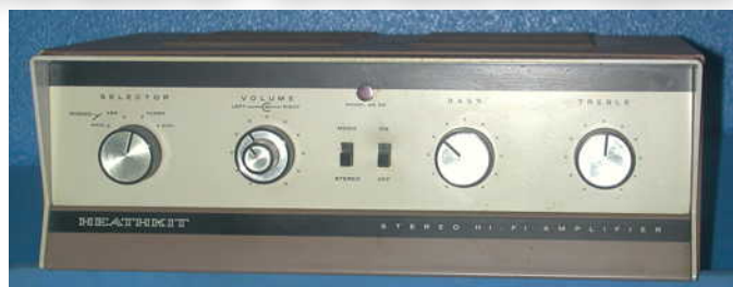
Fig. 1: Heathkit AA-32 Stereo Amplifier
