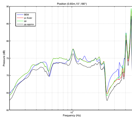
Figure 10: FSM and BEM pressures at the back of the subwoofer
