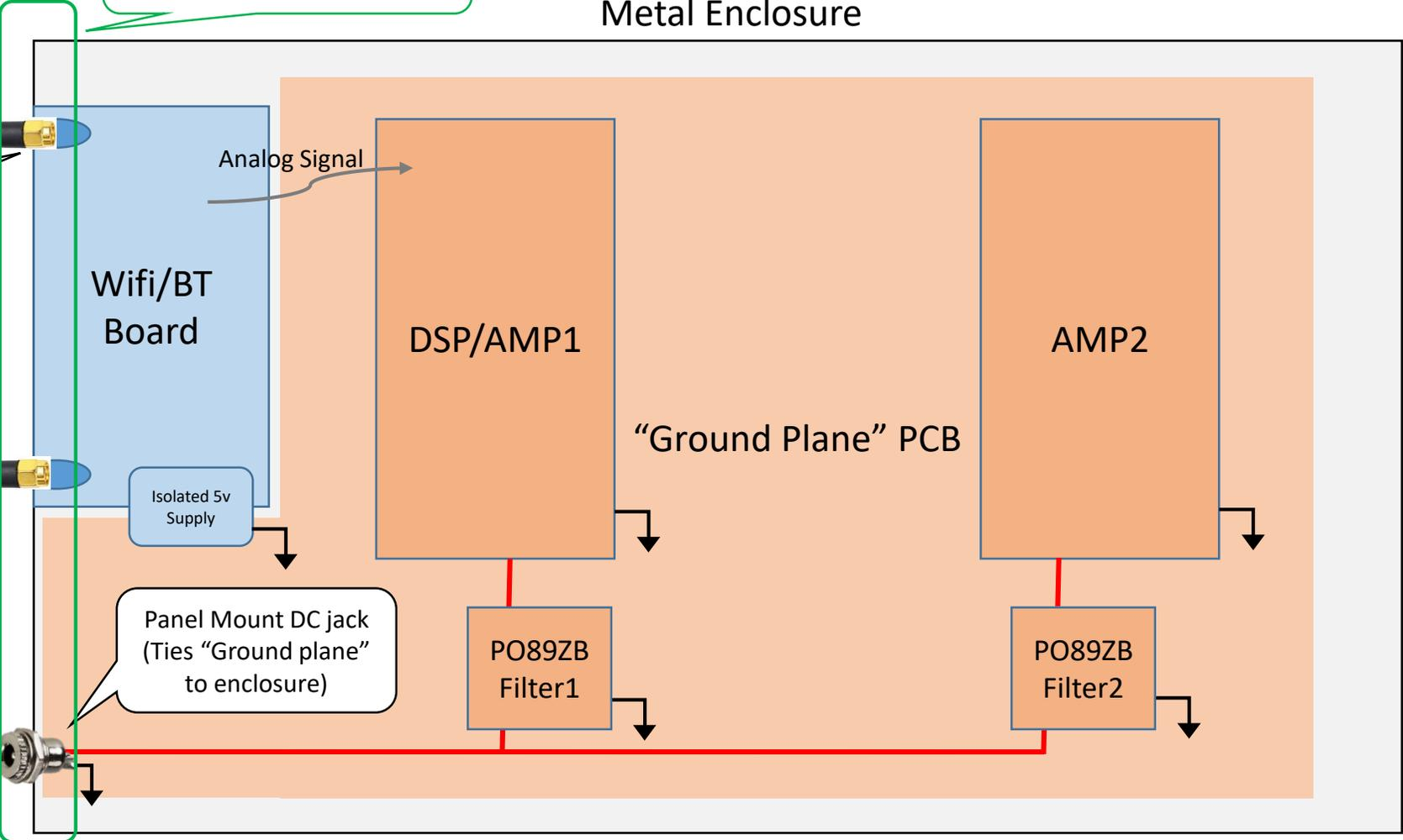
Analog Signal: Single ended, L, R have individual ground wires, joined at DSP/AMP1 – No ground loop noise!
