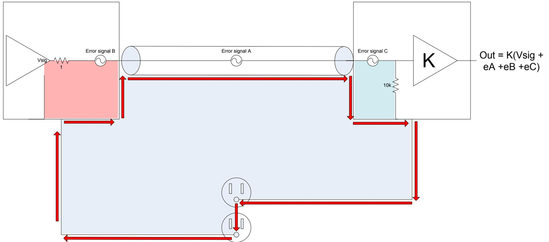
The ground loop current depicted in red is formed by the trapped magnetic flux within the grey loop. The error signal A is the difference between the voltage induced by the trapped flux of the primary loop, minus the flux created by the ground current of the loop. The better the ground, the higher the loop current and the better the cancellation. This means all the ground path, line cords as well as IC's. ( But, it enhances the pink and blue area flux.)
