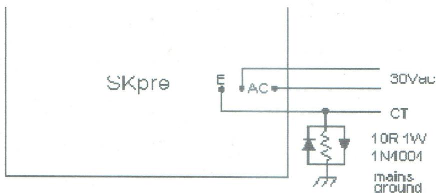
Make sure the transformer regulation is < 15% or use a lower voltage like 24Vac CT if it's greater than 15% regulation, as with smaller ones.
