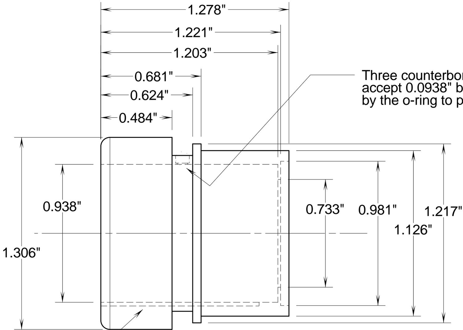
Three counterbores at 120 degrees accept 0.0938" balls that are loaded by the o-ring to provide friction.
